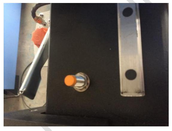
2. The limit switch wire connection ,maybe loose , maybe broken ,please check the wire connection
