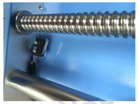
2. The limit switch wire connection ,maybe loose , maybe broken ,please check the wire connection
